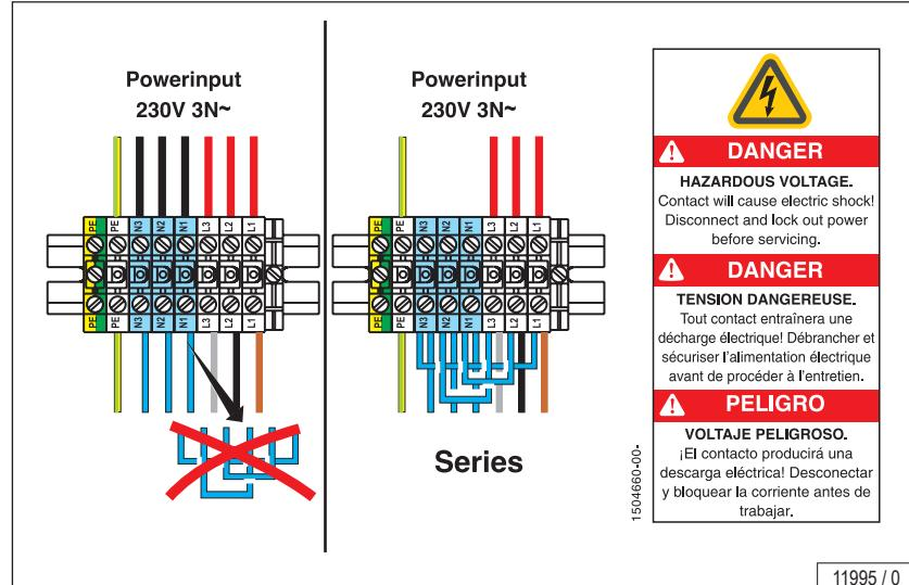
The sticker is visible when the front panel is removed and the control unit cover opened.
